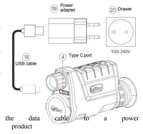
or other USB outlet with a nominal output voltage not exceeding 5 V.
