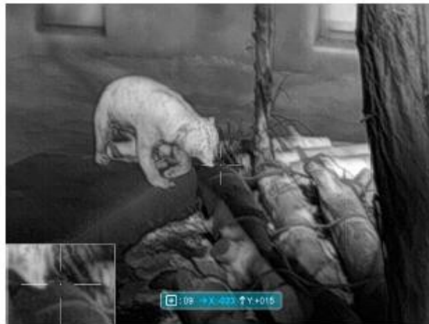
Fig. 6 Defective pixel calibration interface
