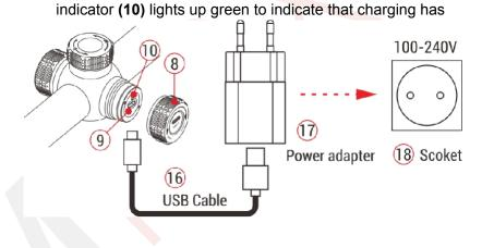
Note: The USB port can only be used to charge the built-in battery.
