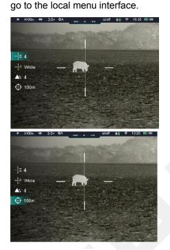
Turn the rotary pushbutton (7) to switch between the following function options, the selected option will be highlighted in the background.
