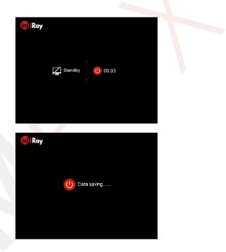
Releasing the button during the countdown puts the device into standby mode. Press the **power button (5)** again to wake up the device.
