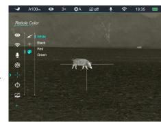
To zero your riflescope, you need to set a zeroing profile and zeroing distance first. Geni LRF Series support the zeroing distance in the range of 1 to 999 m.
